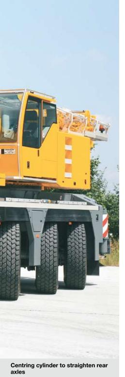
Automatic straightening of rear axles in case of fault
